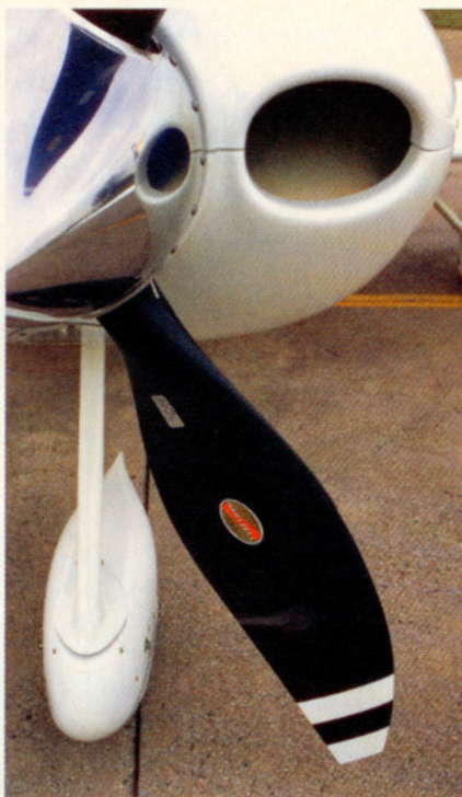
Induction air passes through the filter (above, purple square) before entering the turbocharger scroll through the flexible orange hose. Compressed air is ducted through the white pipe to intercoolers before entering the induction system. Hartzell's second-generation wide-chord advanced structural composite (ASC II) propeller (left) and a built-in 77-cubic-foot oxygen system from Precise Flight (below) are standard equipment on the turbonormalized Cirrus.
